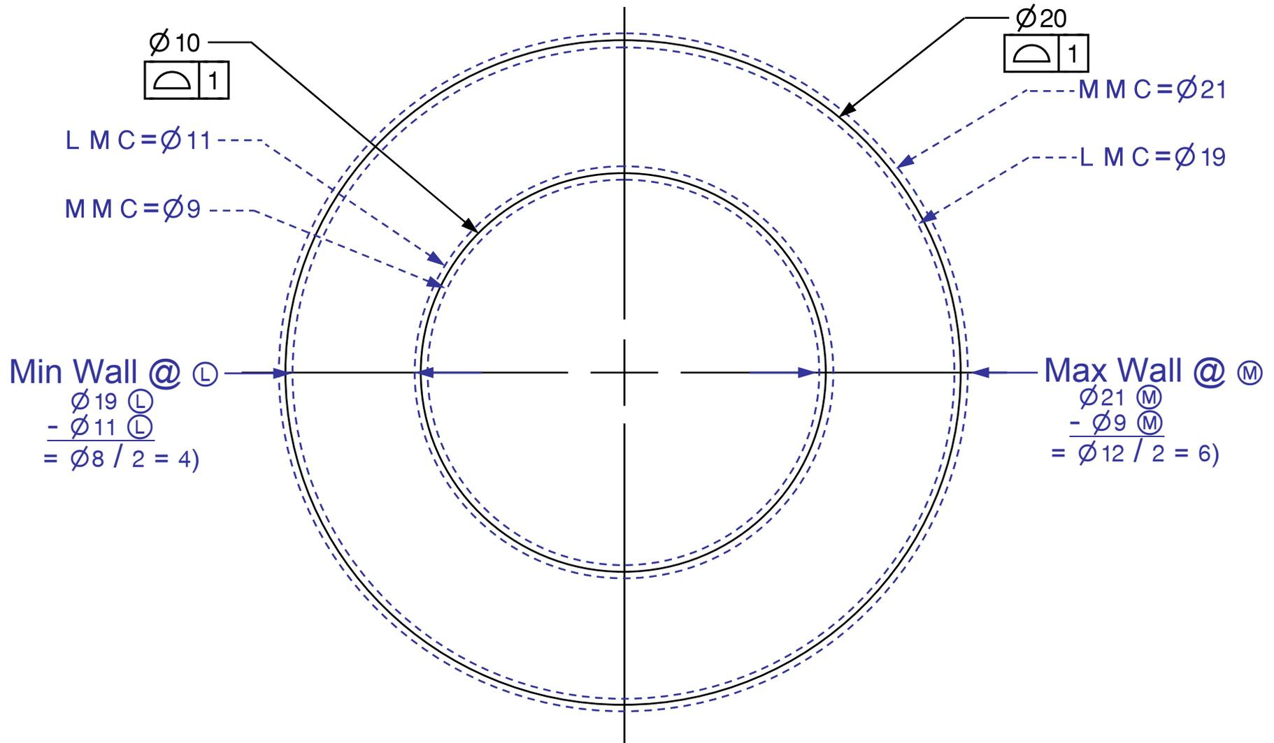
Unless Otherwise Specified All Dimensions are BASIC and controlled Simultaneously
