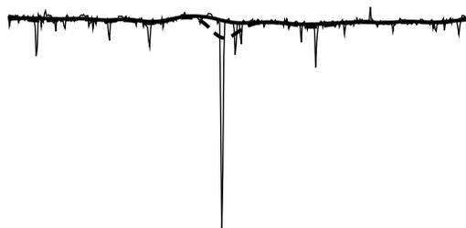
**Figure 22.** Comparison of the mean lines calculated using the non-periodic robust spline filter (solid line) and the Gaussian filter according to ISO 11562 (dashed line) for the profile of a porous surface with the same cut-off wavelength ( $\lambda_c = 0,8$  mm) of both filters.
