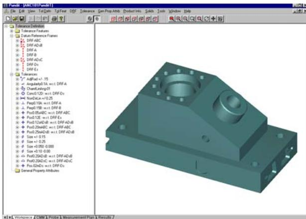
**PUNDIT/CMM workpiece window where parts are imported or created, and checked for tolerancing**
